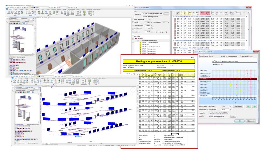
Radiator placement and floor heating
