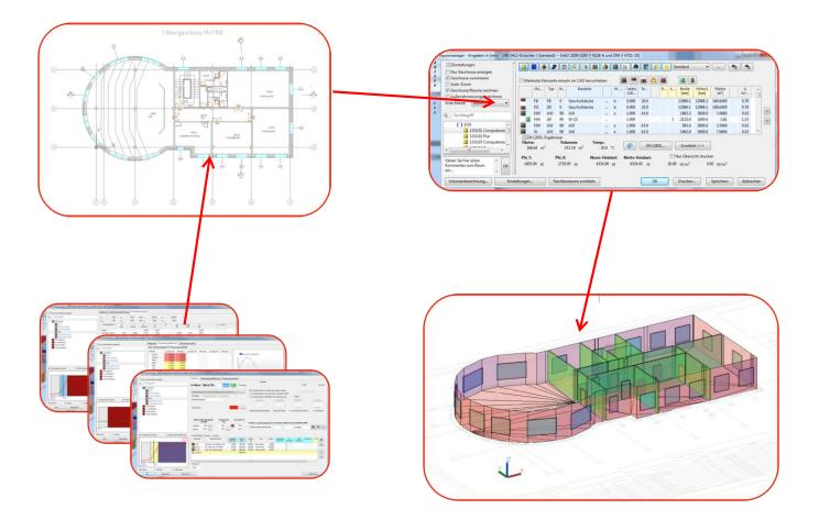
Calculate heating load directly in the CAD system
